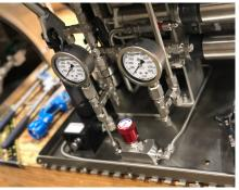
The Sand WASP is suitable for remote locations without the benefit of an available power source such as air, gas or electrical power; and can be used where high concentrations of hydrogen sulfide are present. The Sand WASP can be applied to marginal oil and gas fields that require simple, reliable, low cost system for monitoring pressure, fire and shutdown.
