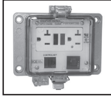
RJ-45 CAT5 F/F connector with 120 VAC Duplex GFCI with internal Simplex GFCI & 3 Amp circuit breaker
